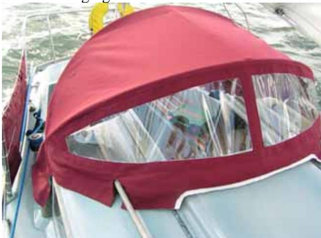
**Slots were cut for the handrail and tape sewn on to reduce wear over the hatch. Press studs were used to fix to roof. Ridgepole prevents puddles.**
