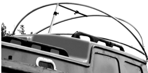
Offering up the frame. The bottom bar rests on the handrails; telescopic stretchers enable you to set the height and pitch you want to end up with
