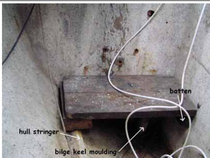
**The box replaced the old battery stowage which was this board at the forward end of the port cockpit locker. It rested on the hull stringer outboard and a batten inboard.**
