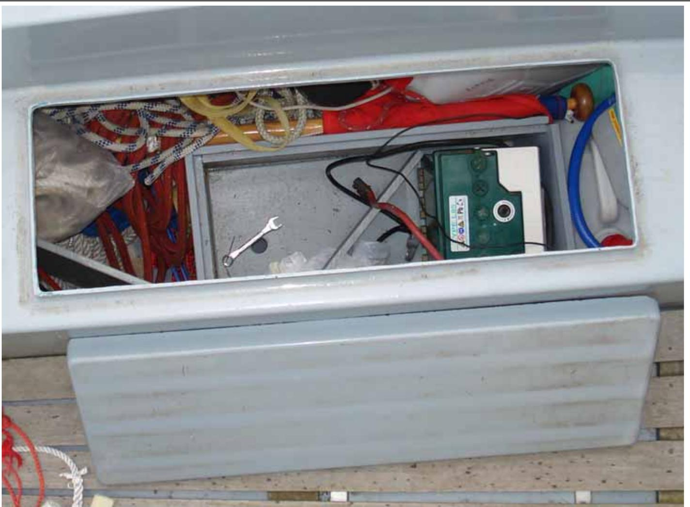
The three sides of the battery box were glassed against the inboard side of the cockpit locker. The floor of the box is a loose fit and sits on the battens provided for this. The lid of the box is not in place in this picture.
