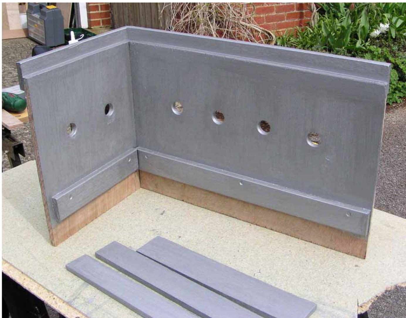
**The battery box was made up by glassing three sides of a box to the inside of the port cockpit locker (2 of the 3 sides seen here). The battens at the bottom are to support the floor (the extra battens beneath were fixed to the locker side). Further battens fixed round the top to create a lip to retain the lid. The bottom edge of the box is not primed as this was to be trimmed and glassed into the hull.**
